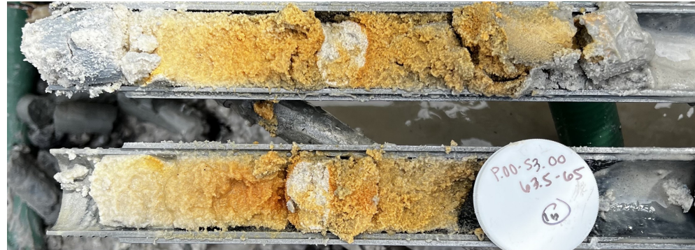
Light brown and orange fine to coarse grained sand with silt (SP-SM)
