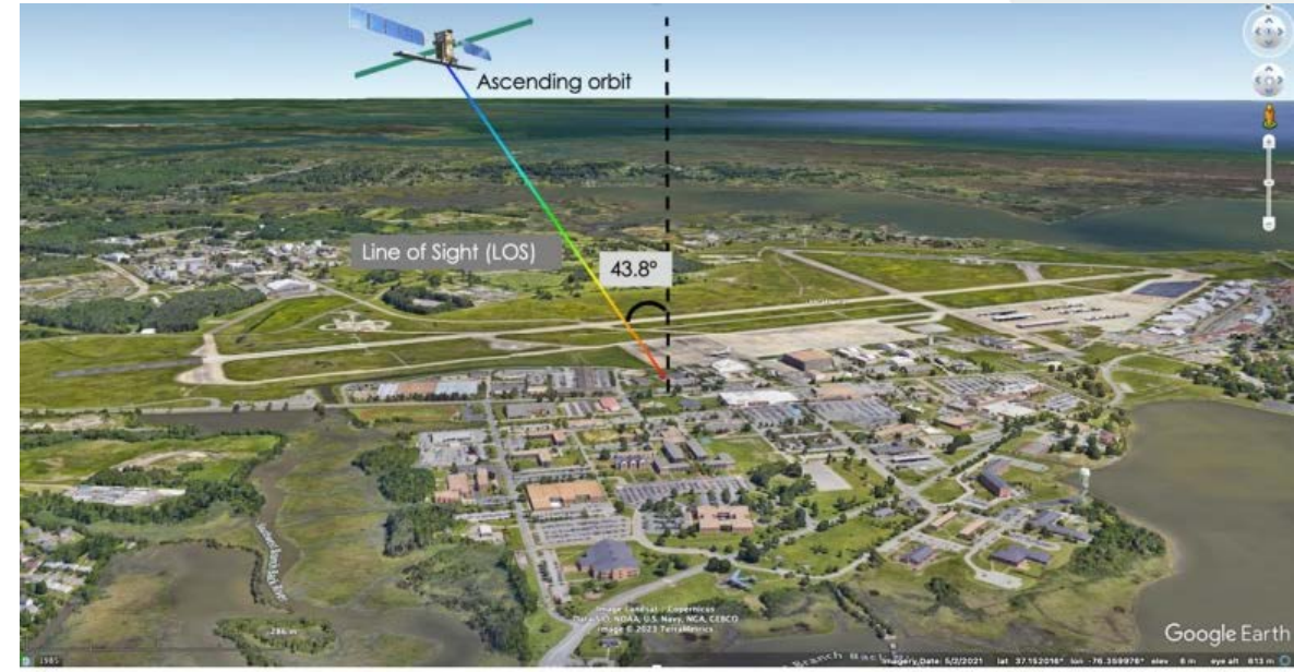
Figure 7 - Geometry of acquisition Ascending orbit in the area of interest.
