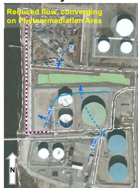
Post-Cutoff Wall July 2013
