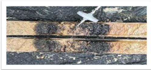
Typical Area 3 NAPL stringer, SB-100 46-47 ft bgs
